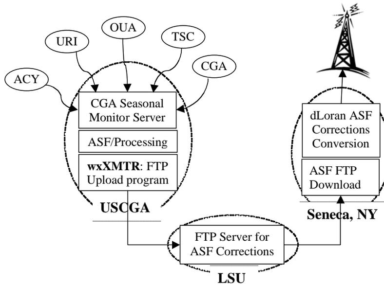
Figure 4: Differential Loran correction data distribution.
