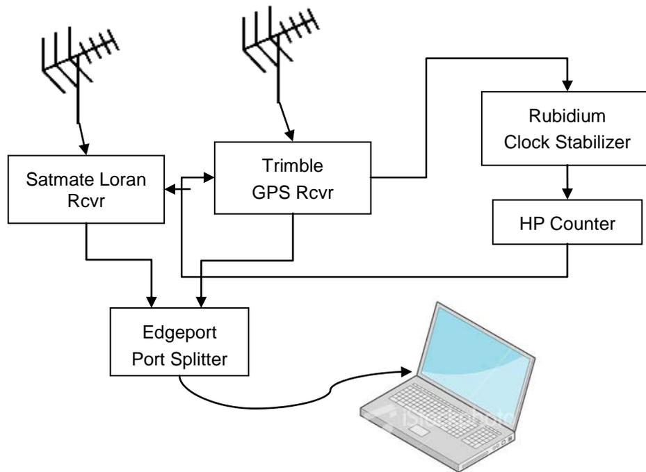
**Figure 3: Block diagram of a Seasonal Monitor configuration.**
